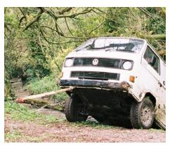
I've already said that the Syncro is built tough. The front recovery point is an example: it's a very nice piece of work, go on, go have a look at it. While you're there check it thoroughly for rust and cracks etc make sure you check the steel around it, too. If you're being recovered from the front it's probably going to be the only thing keeping a very effective missile fixed to your vehicle.
